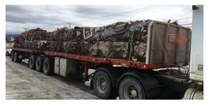
process, without significantly reducing the vehicle's length or width. A cube of miscellaneous crushed metal must be secured by the general cargo requirements.
